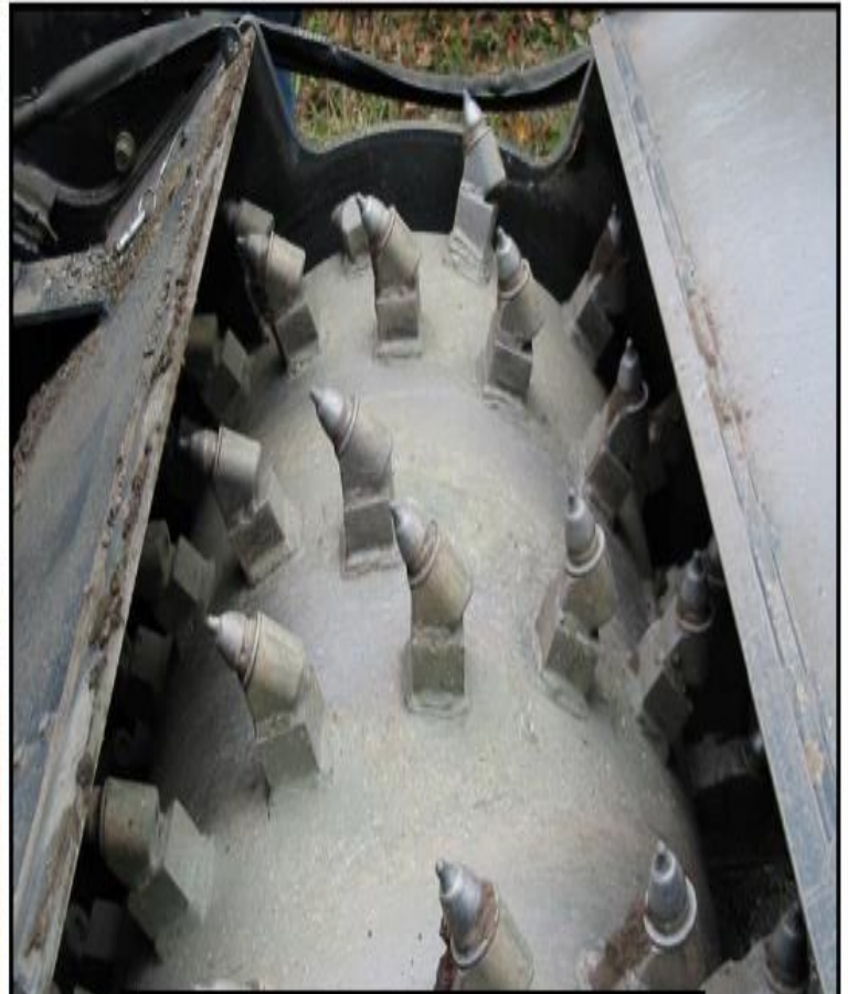
Tooth pattern is optimised for milling or reclamation
